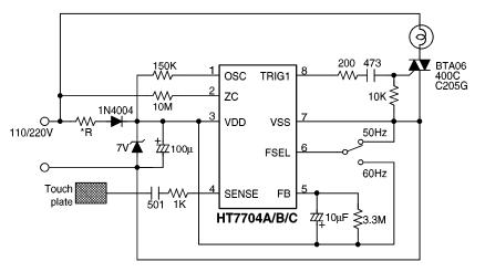
\* Note: 1) R=22K  $\Omega/2W\,$  when the AC power supply is 110V. R=43K  $\Omega/2W\,$  when the AC power supply is 220V.
