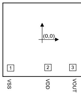
Chip size:  $1111 \times 1051 \text{ } (\mu\text{m})^2$
