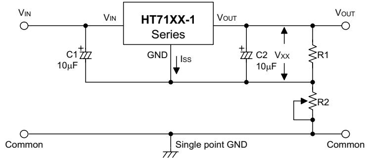
$$V_{OUT} = V_{xx} \left(1 + \frac{R_2}{R_1}\right) + I_{ss} R_2$$
