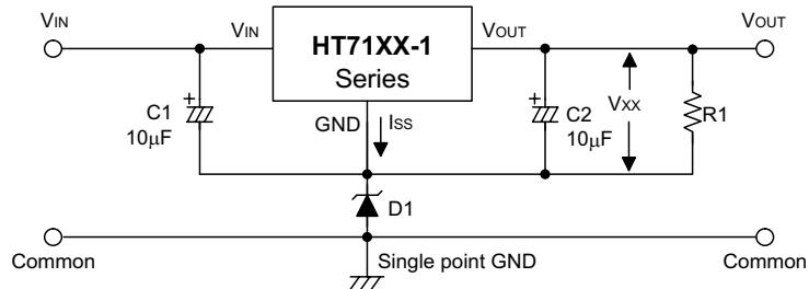
$$V_{OUT} = V_{XX} + V_{D1}$$
