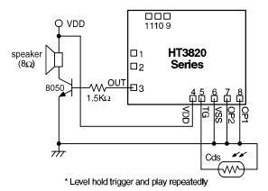
\* Note: The IC substrate should be connected to VDD in the PCB layout artwork.
