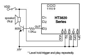
\* Note: The IC substrate should be connected to VDD in the PCB layout artwork.
