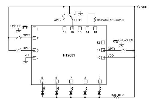
\* The IC substrate should be connected to VDD in PCB layout artwork.
